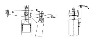
inductive proximity switch "brake closed" as per WN 200/55 with sensor Bi5-M18-AZ3X
