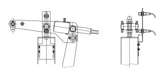
inductive proximity switch "pad wear limit" as per WN 200/04-1 with sensor Bi5-M18-RZ3X
