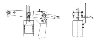
inductive proximity switch "open & closed" as per WN 200/56 with sensor Bi5-M18-AZ3X
