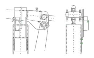
mechanical twin limit switch "open & closed" as per WN 200/53 with switch Z4VH336-11z
