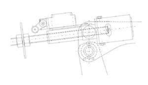
emergency manual release with mechanical limit switch ZR336-11z for indication "manual release engaged" as per WN 200/03
