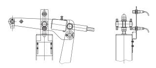
inductive proximity switch "pad wear limit" as per WN 200/04-1 with sensor Bi5-M18-RDZ3X
