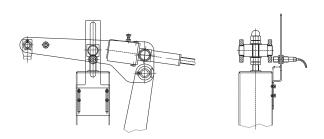
inductive proximity switch "open & closed" as per WN 200/56 with sensor Bi5-M18-ADZ3X
