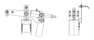
inductive proximity switch "brake closed" as per WN 200/55 with sensor Bi5-M18-ADZ3X
