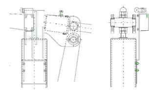
mechanical limit switch "brake closed" as per WN 200/52 with switch PS316-Z11-H310-U2
