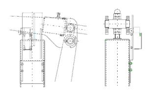
mechanical twin limit switch "open & closed" as per WN 200/53 with switch PS316-Z11-H310-U2
