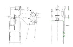
mechanical limit switch "pad wear limit" as per WN 200/04 with switch PS316-Z11-H310-U2
